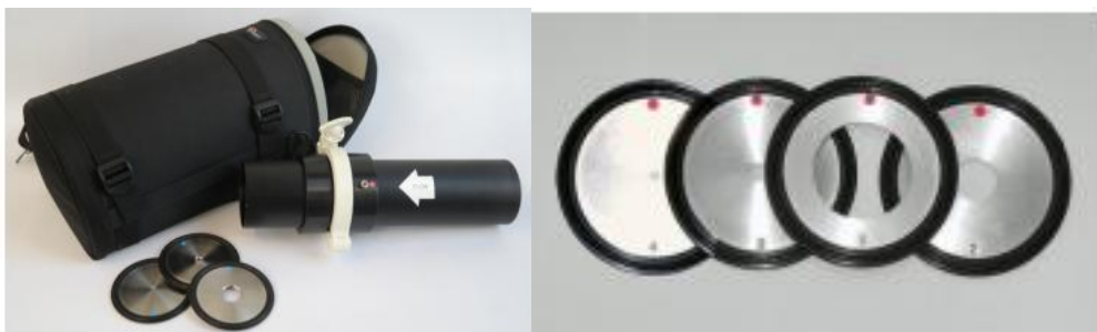
Figure 43 Micro Leakage Meter (MLM) and 4 disks with different size of opening diameter
