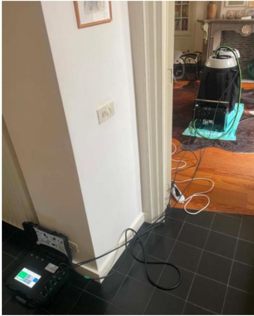
Figure 19 Setup of pressure vessel and controller to avoid direct interaction
