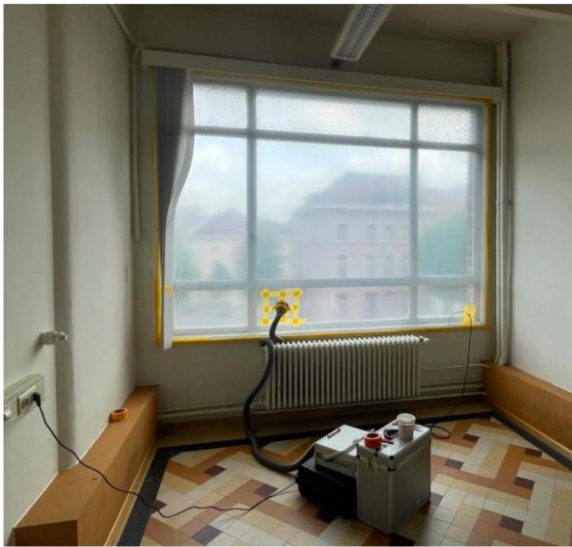
Figure 24 On site testing of window airtightness using Lindab duct testing equipment
