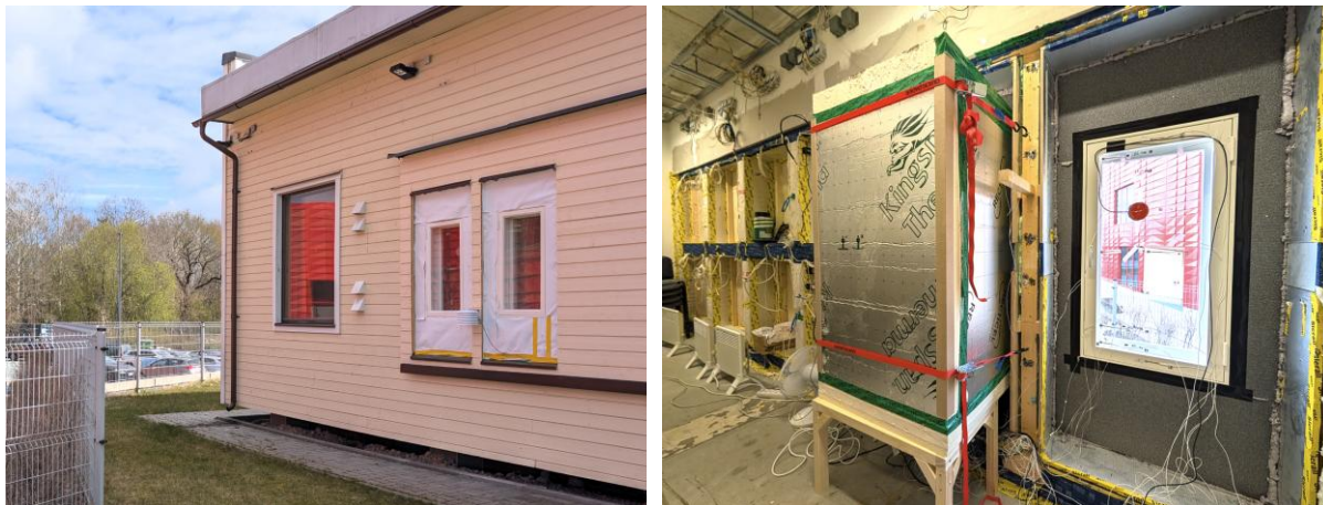
Figure 34 Windows being tested in the nZEB Test Building of TalTech. Photo from the outside (left) and inside (right): hotbox can be seen installed on the left window, heat flux and temperature sensors are visible on the rightmost window.
