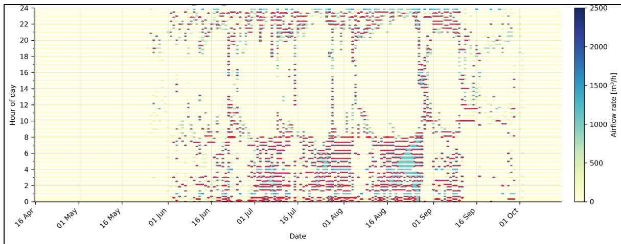
Figure 18: Hourly distribution of AFN-predicted inflow airflow rates in the second-floor kitchen as a function of day of year and hour of day. The red contour identifies the airflow requirement of 830 m 3 /h; regions within the contour correspond to periods when the required ventilation rate is achieved
